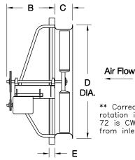
\*\* Correct propeller rotation is CCW (size 72 is CW) when viewing from inlet side.
