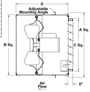
Note: Correct propeller rotation is CCW when viewing from inlet side.
